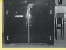
outside skins together is specially constructed to minimize heat transfer from the inside to the outside panel. These panels are commonly filled with #4 pound insulation and are spot welded construction, 4" thick, and consist of #20 gauge satin coat sheet steel inside and outside.
